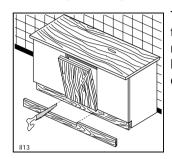
To allow correct opening of the door it is sometimes necessary to cut the kitchen plinth. Refer to the cutting table below.
